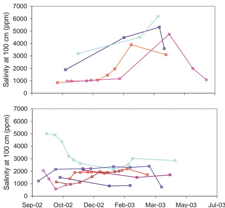
**Figure 7. Trends in salt concentration for selected sites. Rising trends at 100 cm are shown in the top chart and steady or falling trends in the lower chart.**
