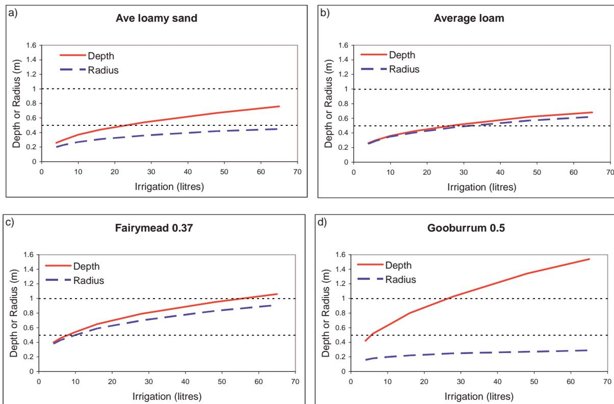
**Figure 5. The depth (solid line) and radius (dashed line) we expect water to penetrate for a given amount of irrigation from a dripper in four different soil types. In each case the initial conditions were relatively dry (100 kPa).**
