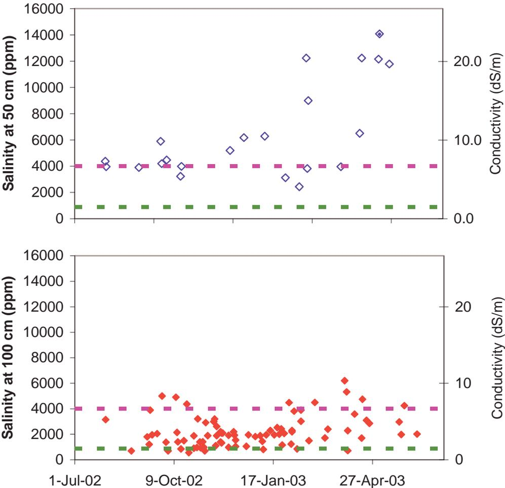
**Figure 6. The salinity of water (left axis in ppm and right axis in dS/m) collected from the 50 cm FullStops (top) and 100 cm FullStops (bottom). The lower dotted line shows where yield starts to decline and the upper dotted line where yield could be reduced by 50% according to Mass and Hoffman 1977.**
