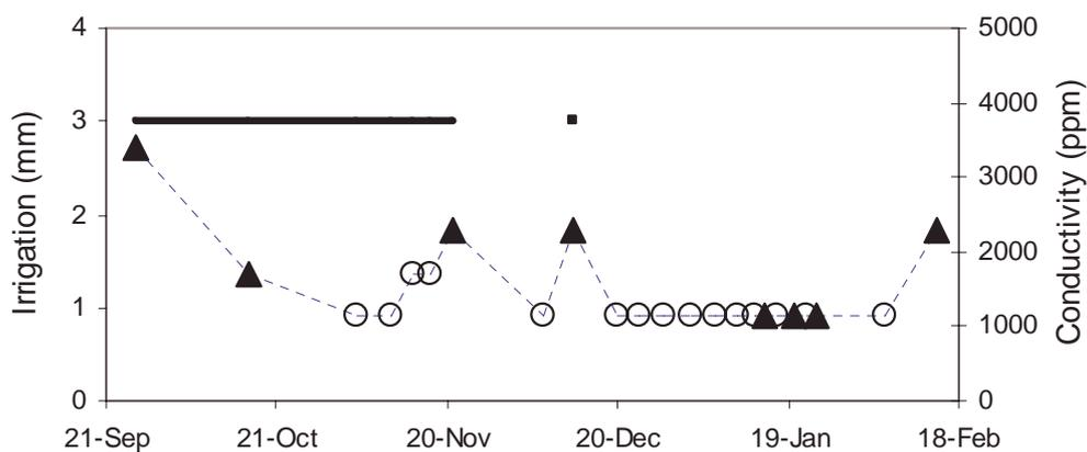
**Figure 12.** The graph plots the amount of irrigation water applied via drippers at each irrigation date. The marker for each irrigation day is an open circle if no detector was activated and a filled triangle if the 50 cm deep detector was activated. The solid horizontal line shows the period when the LongStop contained water.
