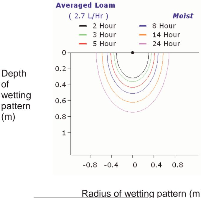
**Figure 4. An example from “WetUp” showing the radius and depth of a wetting front 2, 3, 5, 8, 14 and 24 hours after irrigation commenced from a 2.7 l/h dripper. The simulation shows that it would take around 8 hours for a wetting front to reach a depth of 0.5m, even starting from a moist soil. According to the model the irrigation system would need to be run for over 24 hours to activate a 1.0m deep detector.**
