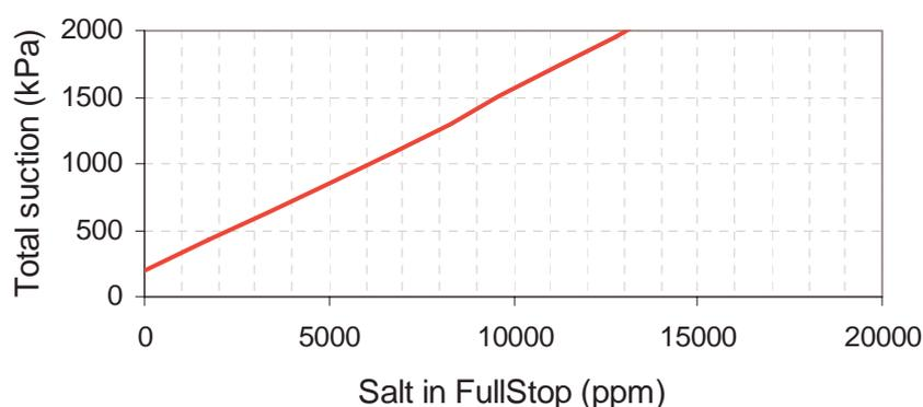
**Figure 9. The total suction experienced by the vine as a function of the salt concentration recorded in the FullStop when a gypsum block reads 200 kPa.**
