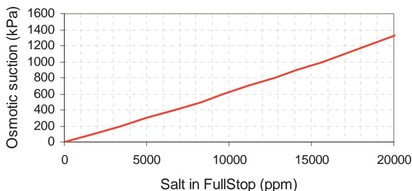
**Figure 8. The relationship between the salinity of the water and the osmotic suction experienced by the vine roots. The above example assumes all the salt is NaCl<sup>6</sup>.**
