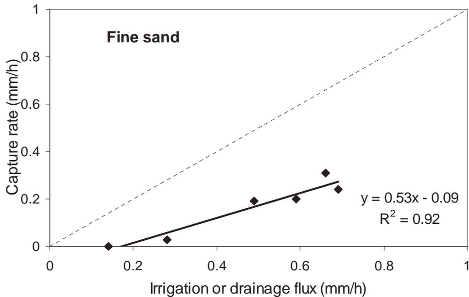
**Figure 11.** The rate that water is moving past the detector (irrigation or drainage flux) compared to the rate water is captured at the base of the funnel for a fine sand. The dotted line represents the 1:1 ratio where the capture rate equals the drainage rate.
