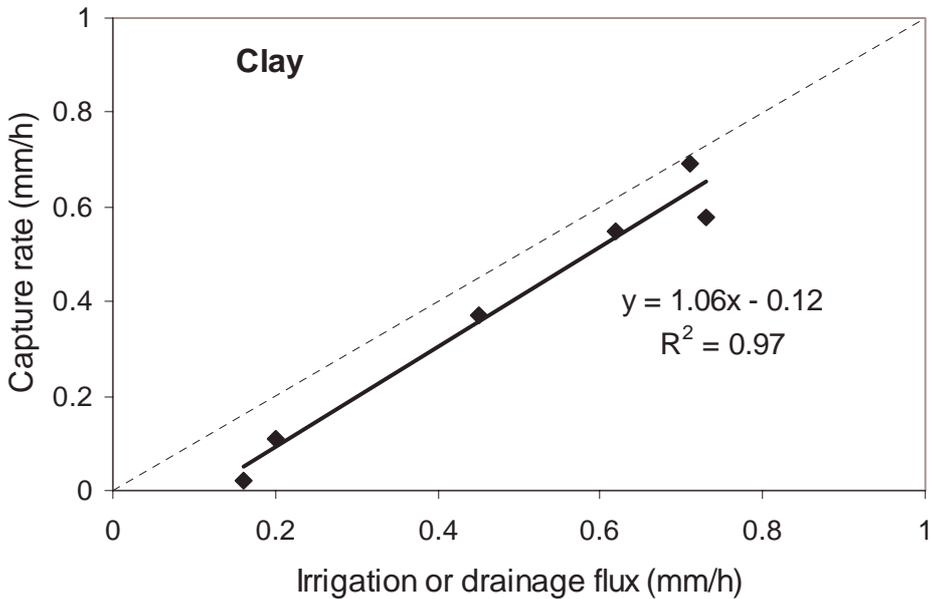
Figure 10. The rate that water is moving past the detector (Irrigation or drainage flux) compared to the rate water is captured at the base of the funnel for a clay soil. The dotted line represents the 1:1 ratio where the capture rate equals the drainage rate.
