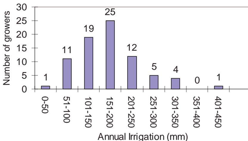
**Figure 1. The total annual irrigation and number of growers in each group for winegrapes under drip irrigation**
