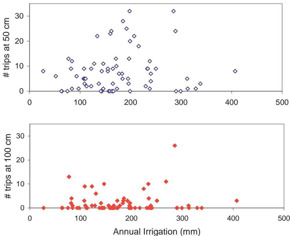
**Figure 3** The relationship between total amount of water applied throughout the 2002-3 season and the number of times the FullStops responded at 50 (top) and 100 cm depths (bottom). Each marker on the graphs represents one grower, showing the annual irrigation applied and the number of times (#) a wetting front was recorded at 50 and 100 cm (72 growers).
